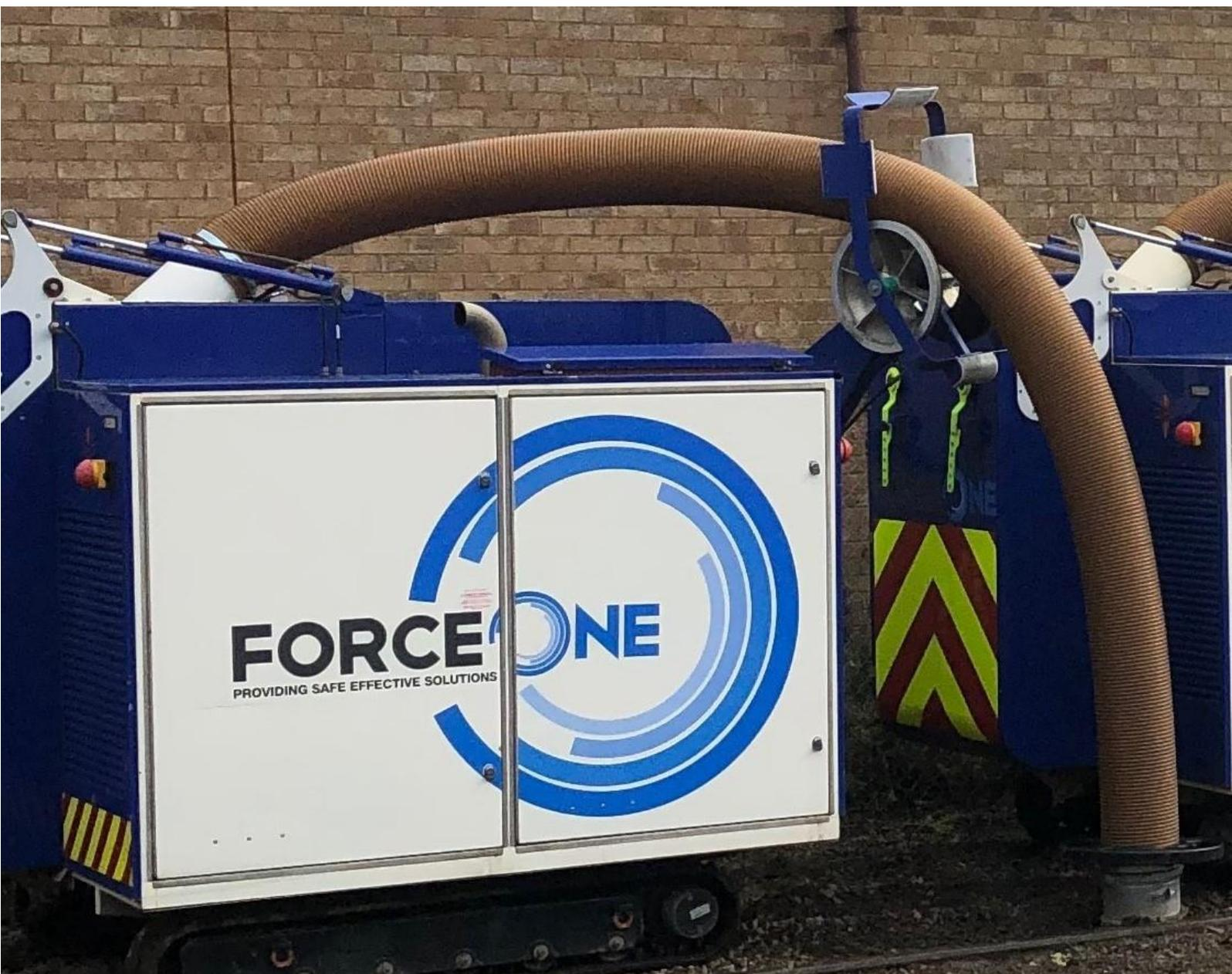
Unique to Force One Ltd, the iVac is a state-of-the-art, remote-controlled, compact track mounted Suction Excavator. The iVac is specially designed for use in projects which involve sensitive service excavations that are limited in size or difficult to access, such as off-road locations, in fields or in built-up areas where other excavators simply cannot reach, such as narrow roads or passages.
